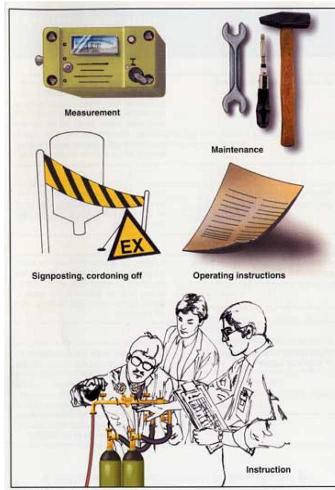
Figure 4.1: Examples of organisational explosion protection measures [From the ISSA leaflet "Gas Explosions", International Section for the Prevention of Occupational Risks in the Chemical Industry, International Social Security Association (ISSA), Heidelberg, Germany]
