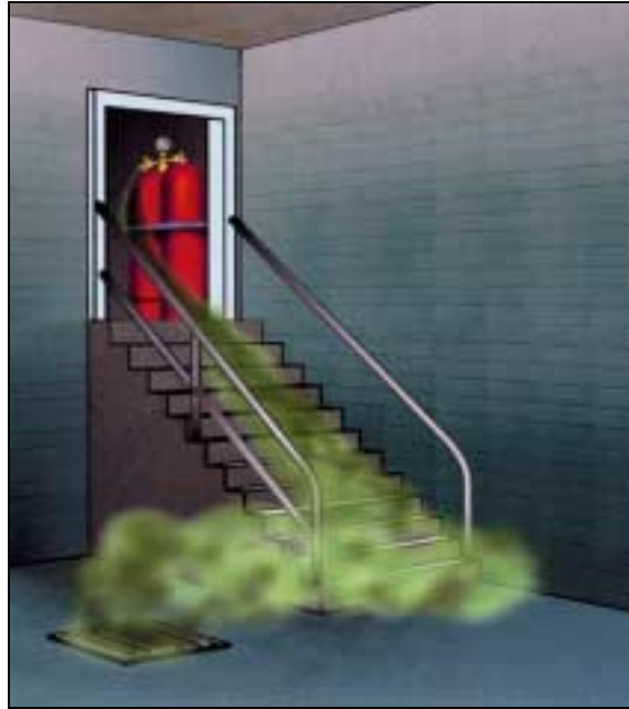
Figure 2.3: Spread of liquefied gases (example) [From the ISSA leaflet "Gas Explosions", International Section for the Prevention of Occupational Risks in the Chemical Industry, International Social Security Association (ISSA), Heidelberg, Germany]
